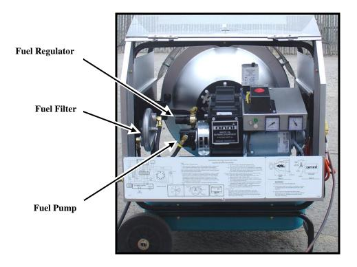
Figure 7 - Radiant Heater (Back View)
