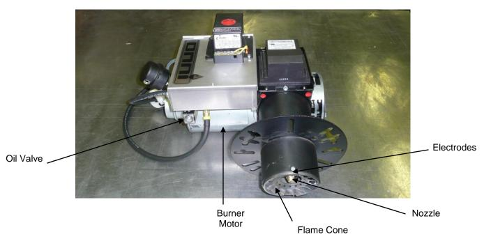
Figure 6 – Oil Burner (Front View)
