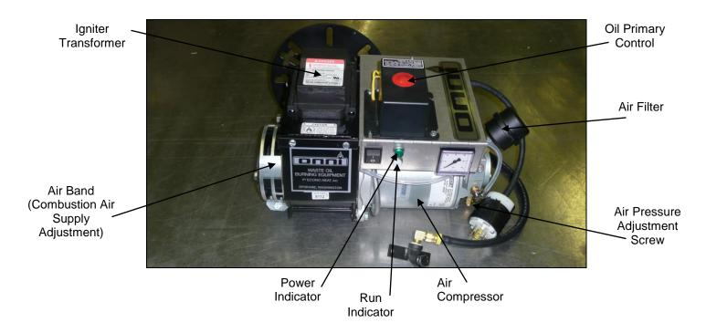
Figure 4 - Oil Burner (Back View Closed)
