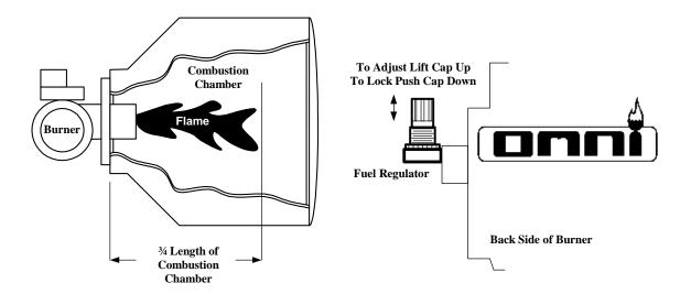
Figure 8 - Flame Adjustment
