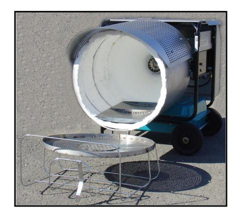
Figure 15 – Combustion Chamber Cleanout Door
