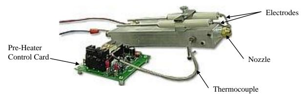
Figure 12 – Pre-Heater Block Detail (Removed From Burner for Clarity)
