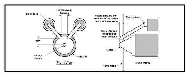
Figure 11 - Electrode Adjustment Detail
