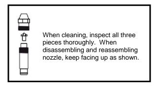
Figure 10 - Nozzle Assembly Detail
