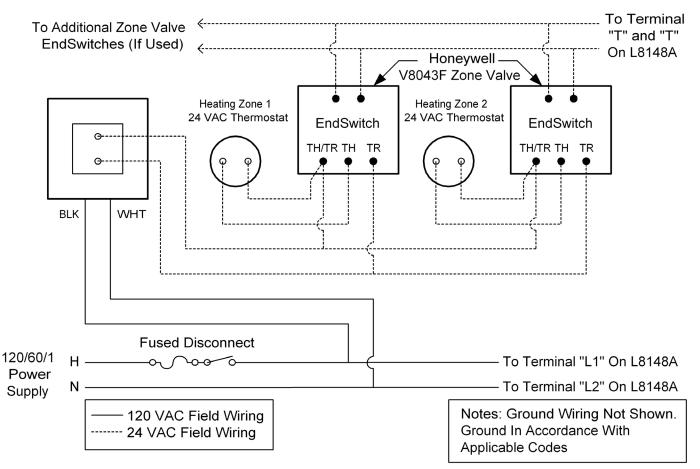
**Figure 23** – Wiring diagram, circulator zone wiring using Honeywell R845A valves (factory boiler wiring not shown here – see figure 21)
