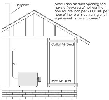
\*If the equipment room is located against an outside wall and the air openings communicate directly with the outdoors, each opening shall have a free area of not less than one square inch per 4,000 BTU per hour of the total input rating of all equipment in the enclosure.
