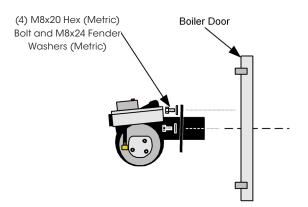
Figure 20 - OWB-9 and OWB-15 chamber swing door burner mounting
