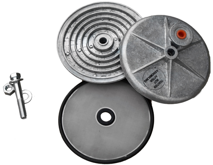
Figure 11 - Oil Filter (Pancake Style Filter)
